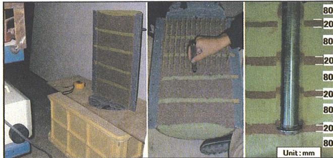
Fig.5 Measurement situation by thermography (left), hardness examination (center) and the position of a layer position situation
