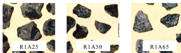
Fig.2 Section photograph of recycled coarse aggregate.
