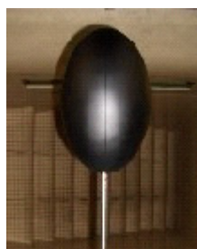
Fig.13 Wind tunnel model based on elliptic shaped body
