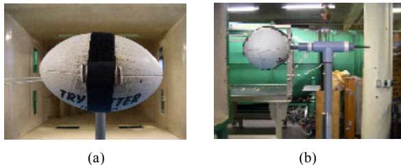
Fig.7 Experiment for measuring revolution rate
