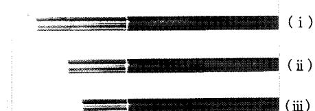
(c) Appearance of machined stepped electrode pipe
