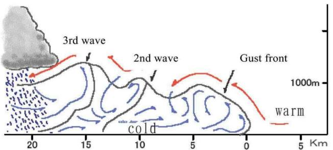
Fig. 13 Outflow of downburst<sup>15)</sup>.
