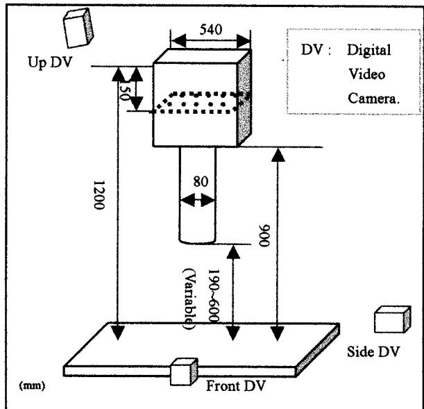
Fig.3 Experimental device.
