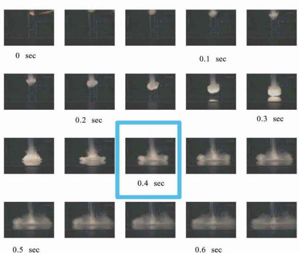
Fig. 4 Serial photos of down-draft (0~0.6sec).
