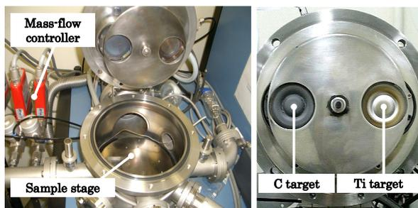
Fig.1 Sputtering system and target
