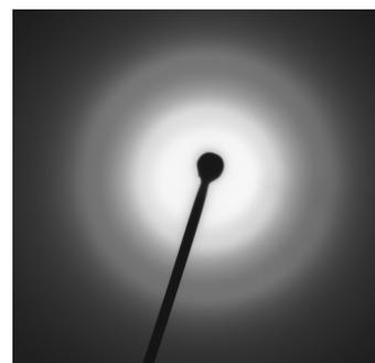
Fig.8 Electronic diffraction image of Ti-doped DLC film
