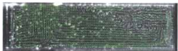
Fig.15 Flow pattern on cross section A in oil strainer model without wire gauze
