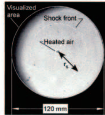
Fig. 2 Visualized laser-induced spherical shock wave (116 \mu s after irradiation).
