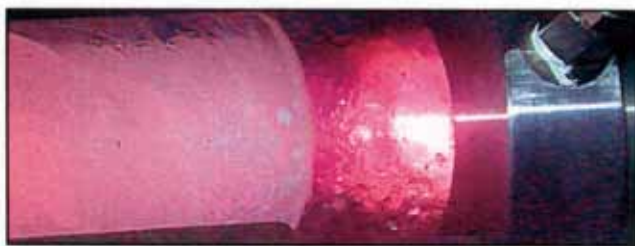
Fig. 18 The rear part of burning fuel
