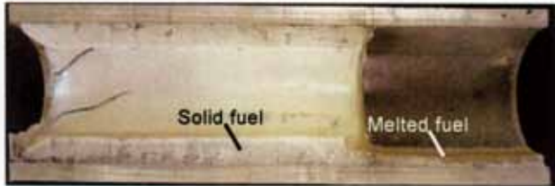
Fig. 16 The cross section of the burnt fuel
