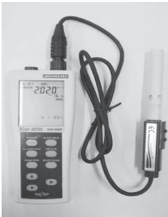
Fig.3 Portable electrical conductivity meter (TOA DKK-HCM-31P)
